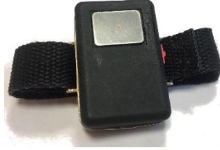
Fig. 1. The ECG WATCH
