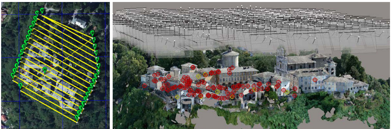
Fig. 5. Example of AAV flight plan over the whole complex and the result of the alignment of the photos acquired.
