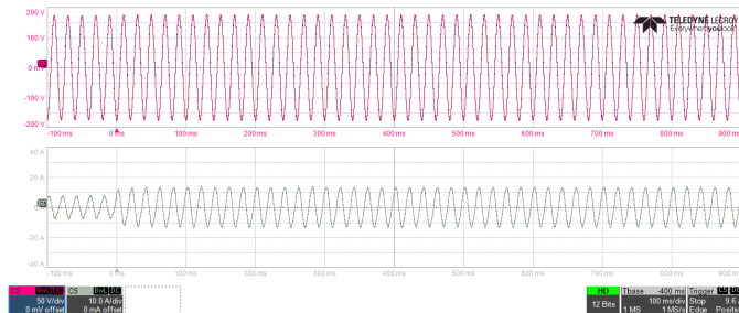
Fig. 17. Test 5: Reactive power reference Q^* step (from 0.1 pu to 0.2 pu). Comparison of VSC operating mode versus VSG/VSCap mode. From top to bottom:
