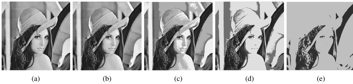
Figure 3: Potential malicious modifications on the truncation parameter ( t ) of approximate logarithmic multiplier (ALM): (a) original result with 8-bit input, (b) t = 6 , (c) t = 4 , (d) t = 3 and (e) t = 2 .
