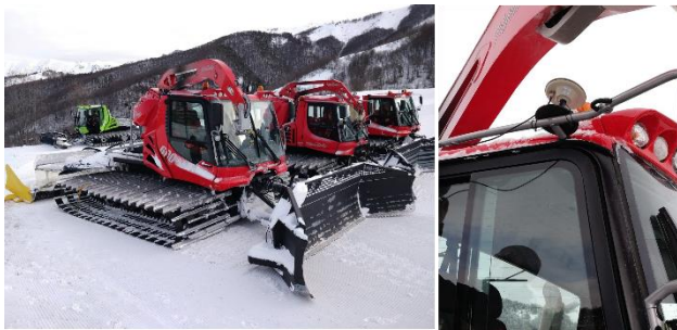
Figure 6. The snow groomer (on the left) and the and the installation of the antenna on the top of the vehicle.
