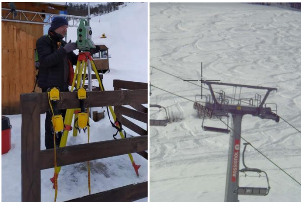
Figure 5. Detail survey with the total station.
