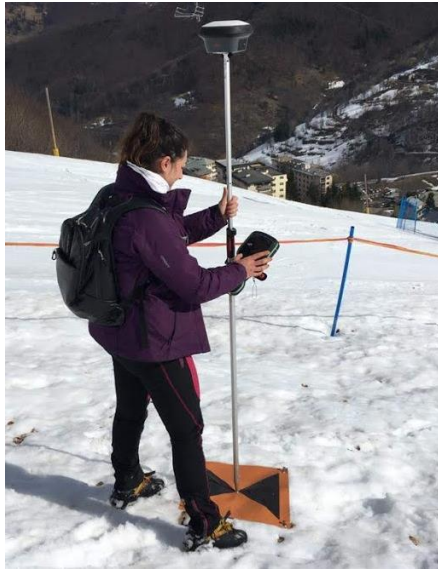
Figure 4. GCPs measurement with RTK approach.
