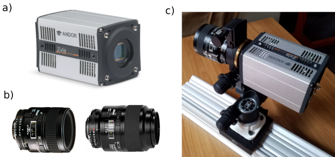
Figure 2.13: Andor Zyla camera (a), Nikon AF 60mm and 105 mm (b) and Camera mounting setup (c). Taken from www.andor.com , www.nikon.com .
