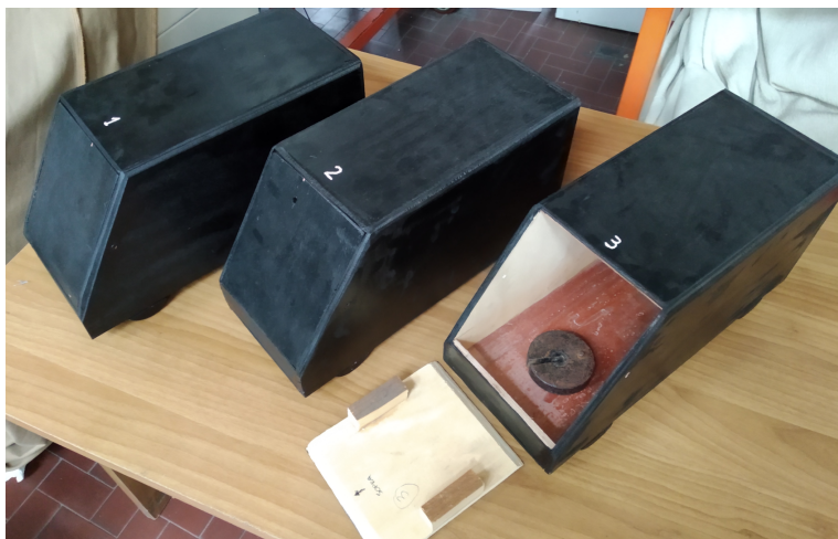
Figure 2.6: The three dummy models numbered. The third one has the slanted front open, where is observable the counterweight within.
