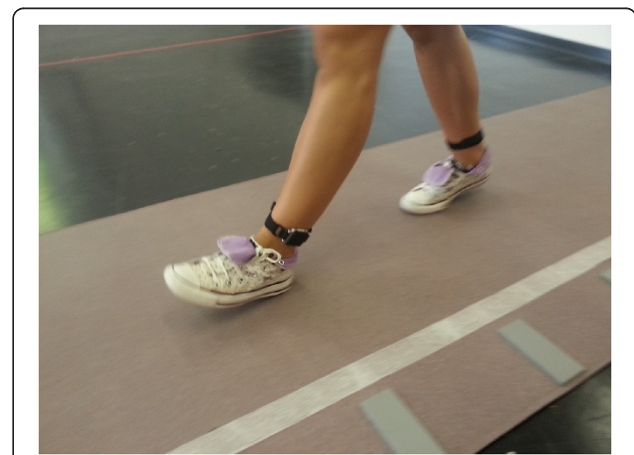
Figure 1 Subject wearing two MIMUs attached above the ankles and walking on the instrumented mat used as gold standard for MIMU based estimates of gait spatio-temporal parameters.
