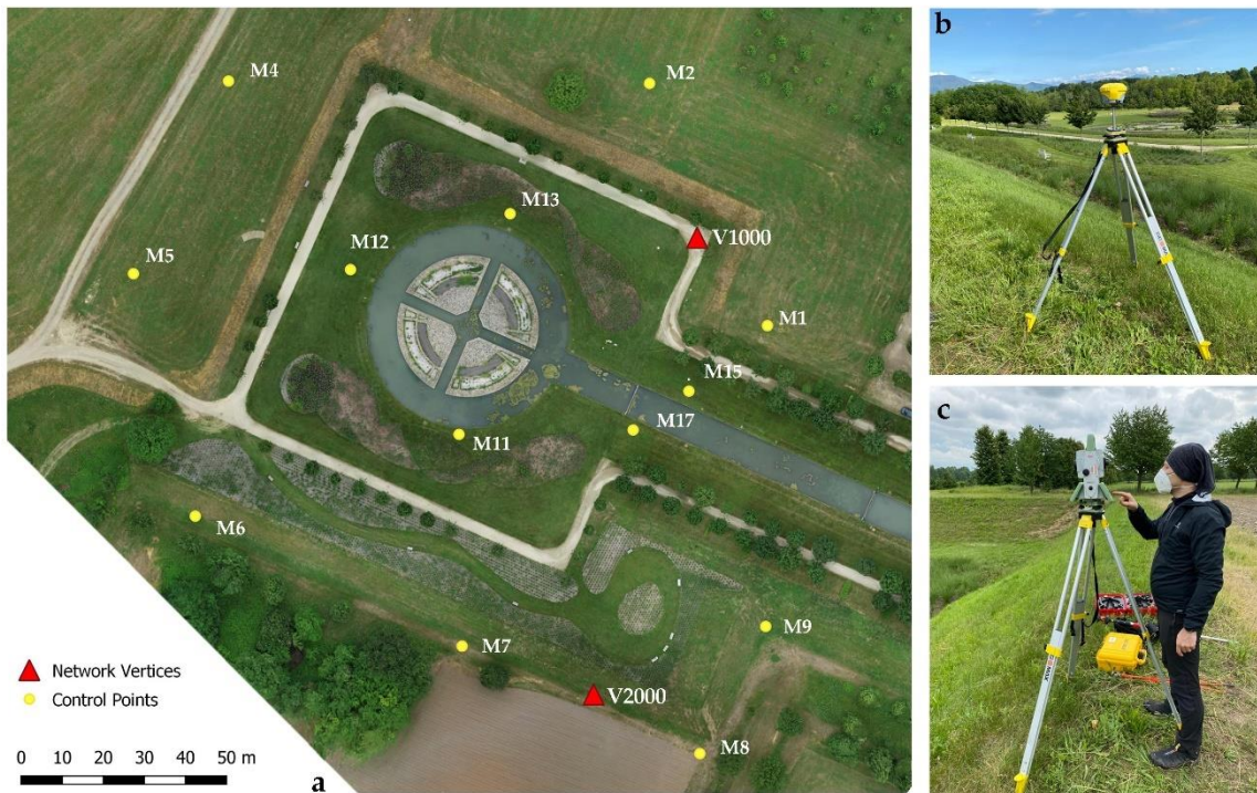
Figure 2. The two vertices of the network (a, red triangles) and the set of control points (a, yellow points). Some of the measurement phases on the field (b,c).
