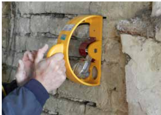
Figure 9. On site rebound test (credits Manuela Mattone)
