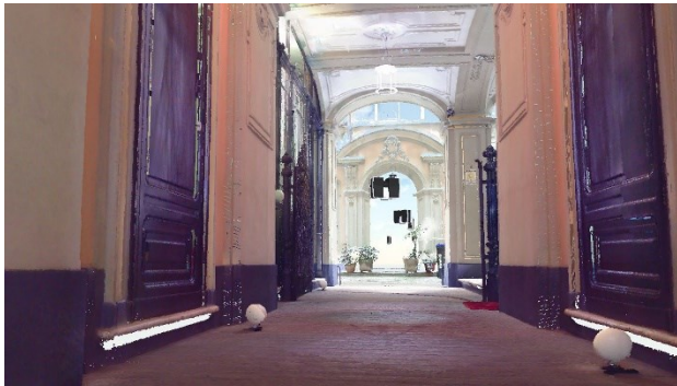
Figure 8. Location of spheres and scan points. Image extracted from the point cloud. Scanning: M. C. López González. Processing: F. Natta
