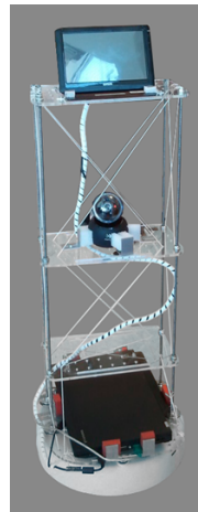
Figure 2. A prototype of the proposed home robot. The system consists of a IRobot Create 2, a laptop computer that was used as a control unit, a Logitech Quickcam Orbit web-camera, and a Mimo Um-720s touchscreen.
