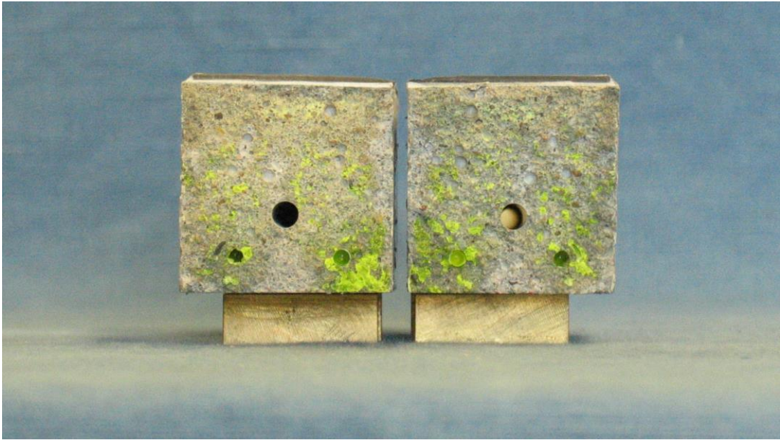
Figure 7.10: Crack faces after splitting of a specimen from the GLASS series.
