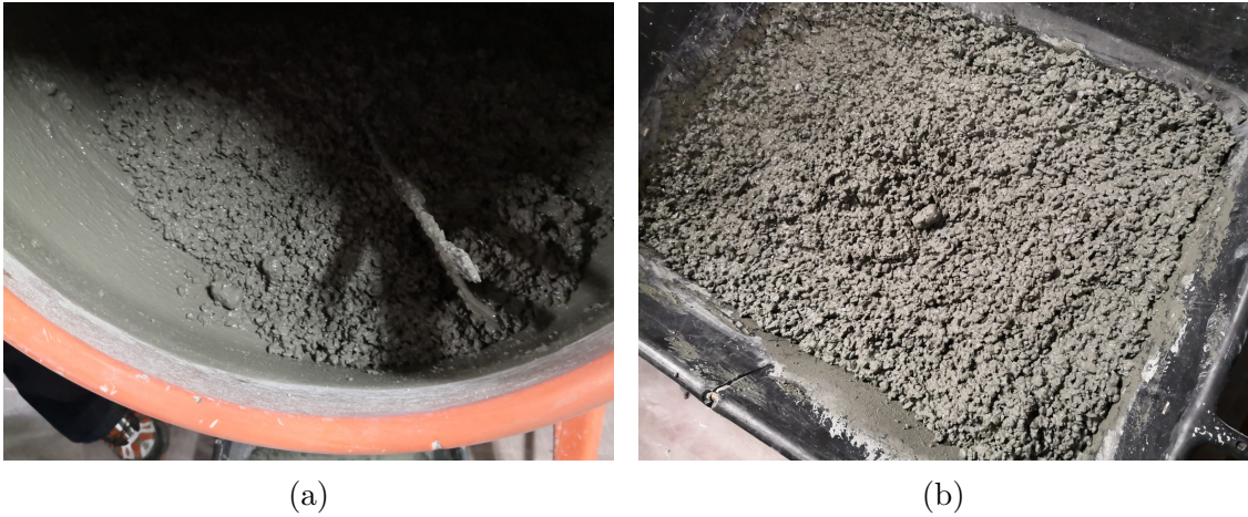
Figure 3.8: Resistance to mixing test: (a) capsules inside the mixer; (b) mix poured in a plastic container in order to retrieve intact and broken capsules.
