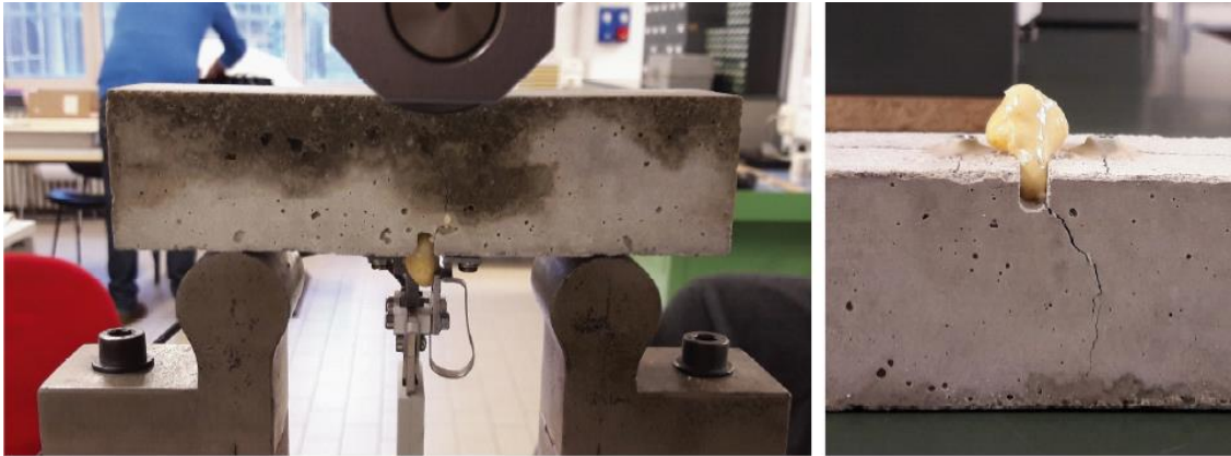
Figure 4.1: Visual observation of the leakage of the polyurethane precursor, causing the formation of hardened polyurethane foam.
