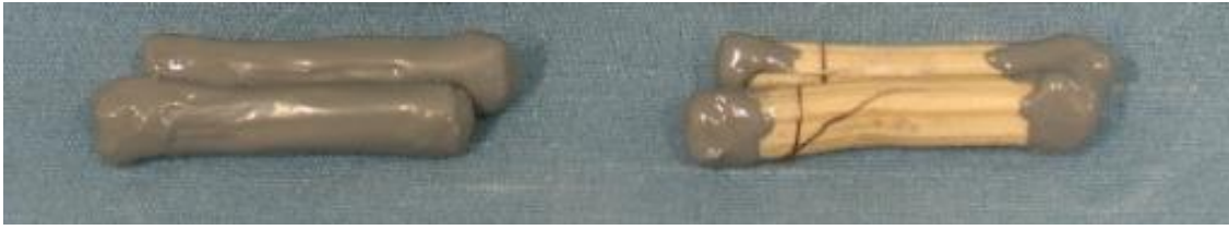
Figure 4.8: Capsules after filling and sealing, either with external or internal coating.
