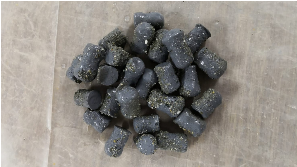
Figure 3.9: Intact capsules after the concrete mixing.
