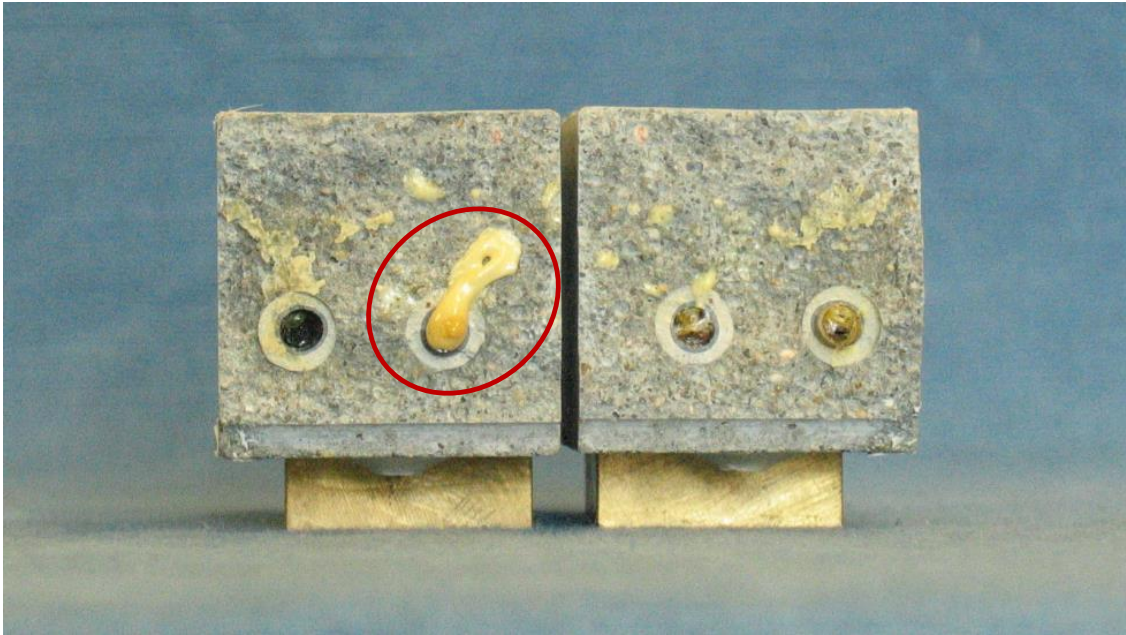
Figure 8.15: Crack faces after splitting of the specimen CEM_B_6. The PU inside the red circle was released after splitting.
