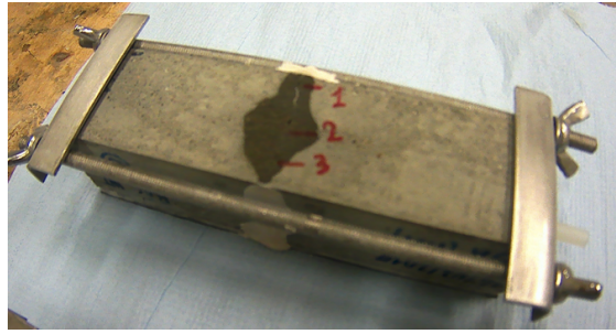
Figure 5.3: Typical sample for which the crack width was controlled using the active crack width control technique. In the figure it is possible to see the healing agent released from the ruptured capsule and spread around the crack mouth (dark colored zone).
