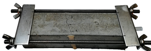
Figure 4. Screw jacks used for actively restraining the crack width of a mortar specimen.
