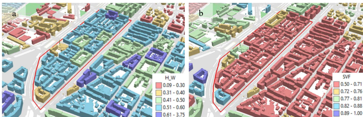
Figure 3. Distribution of the urban variables in a district in Turin: a) urban canyon height-to-distance ratio ( H/W ); and b) sky view factor ( SVF ). The red line outlines the case study area.
