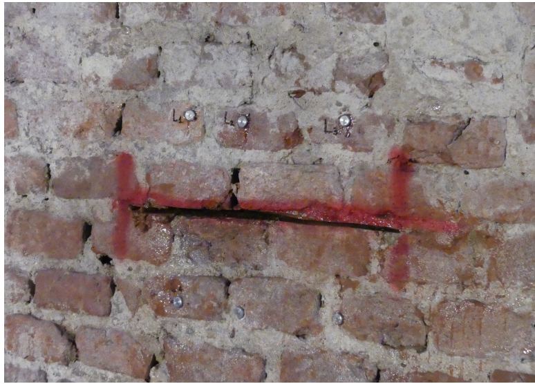
Figure 2.5: The image presents a slot created with a circular saw for the single FJ test. The picture shows also the three couples of measuring points and a thin remaining layer of water used to cool the saw.
