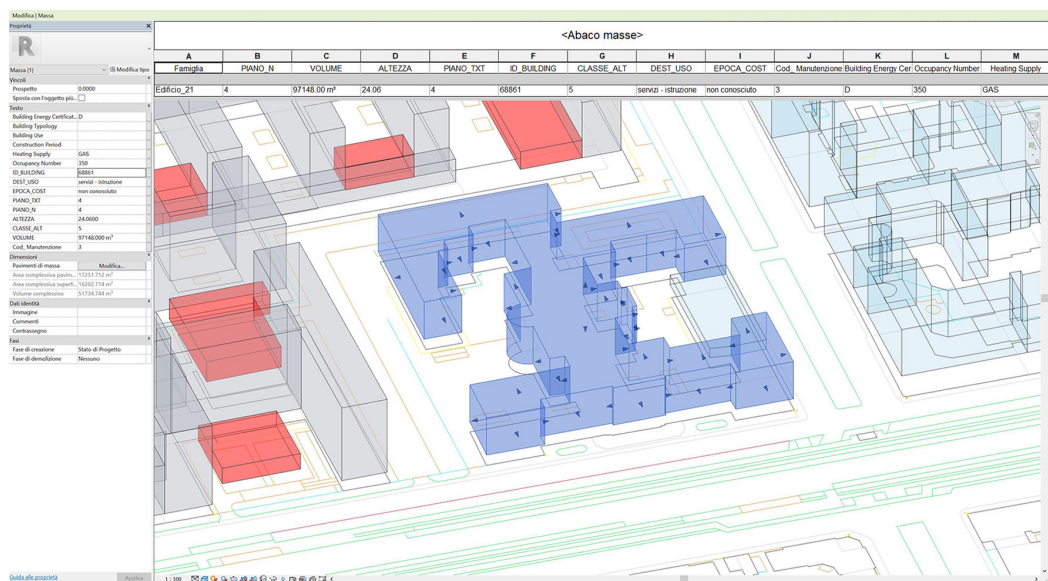
Fig. 2. Geometric and alphanumeric parameters within BIM model.
