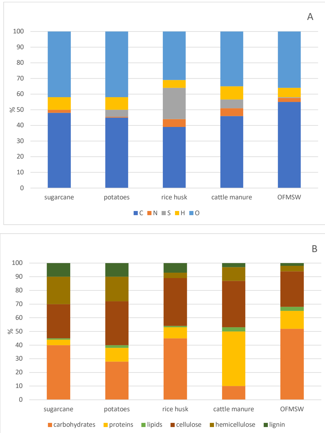
Figure 2. Qualitative description of the selected waste biomasses: (A) elemental and (B) nutritional composition
