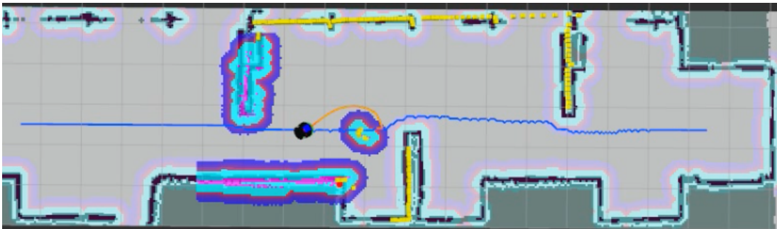
Fig. 8. Test scenario 3: OSGP algorithm reaction to a generic obstacle detection.
