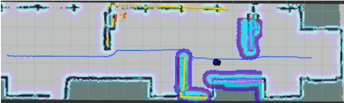
Fig. 7. Test scenario 2: OSGP behaviour when a human obstacle is sufficiently far from the AMR.
