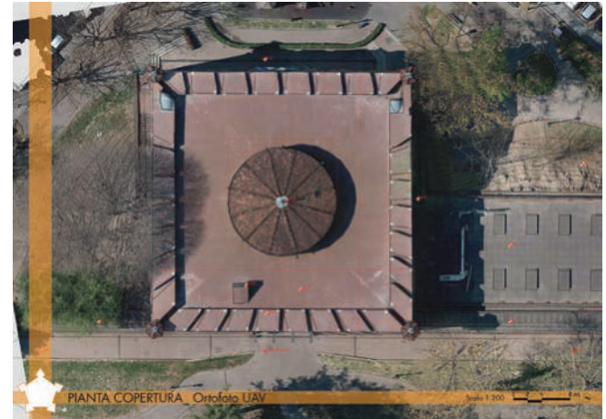
Figure 11. An example of the metric orthoimage derived from the UAVs flights (Group 2: A. Alaimo, A. Bertero, C. Bovet).
