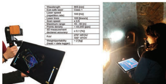
Figure 8. Zeb RT with the connected Tablet (left), technical specification (centre), acquisition phase (right).
