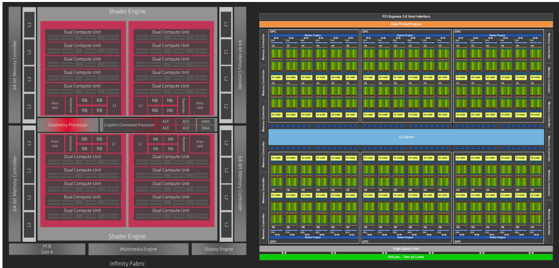
Figure 3.2: Comparison of two architectures available on the market: Navi from AMD and Turing from Nvidia
