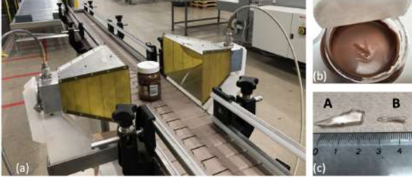
Fig. 14. System set-up for measurements with jars in movement; (a): horn antennas and conveyor belt; (b): example of a contaminant within the hazelnut-cocoa cream jar; (c): considered plastic contaminants.
