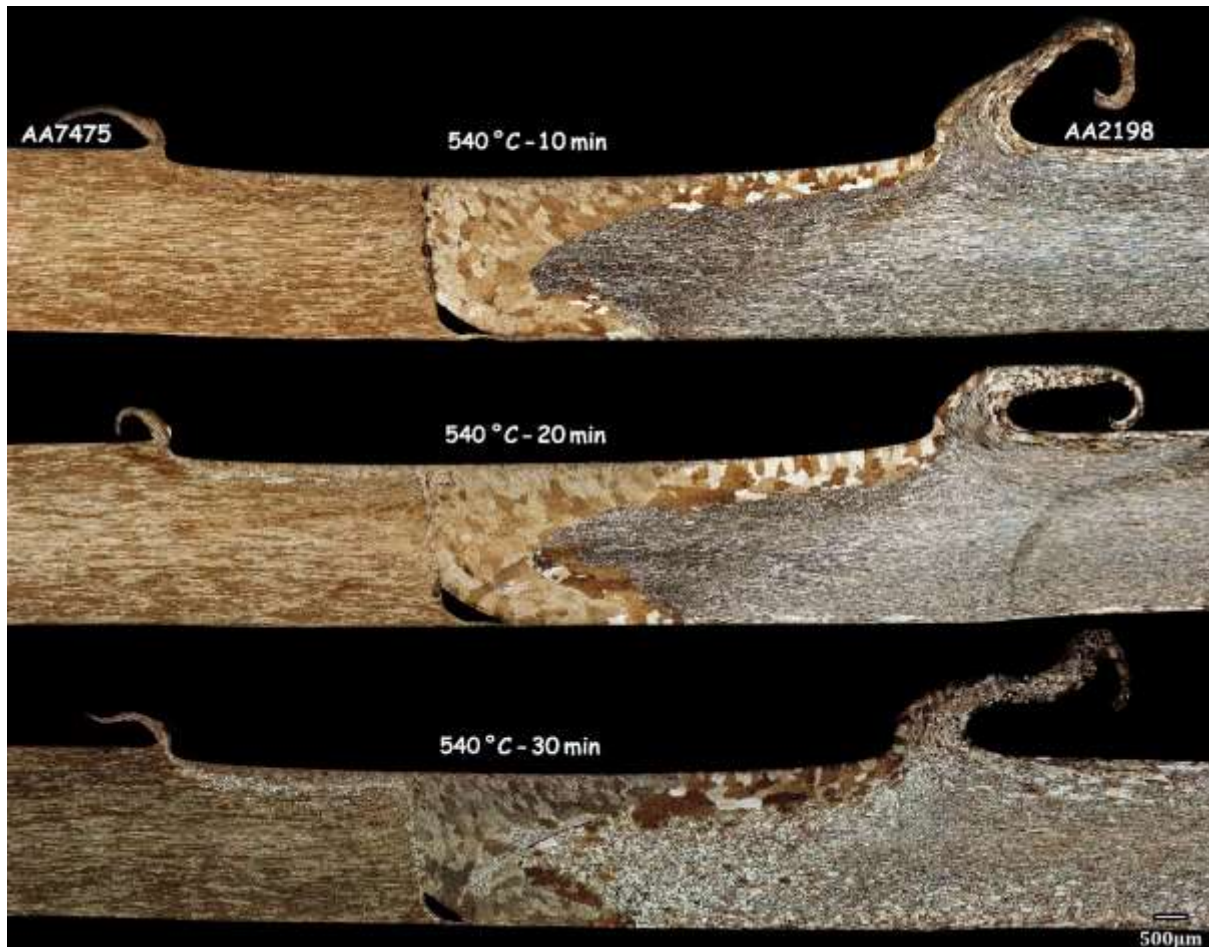
Fig. 13: Solution treatment of dissimilar joint of AA7475-AA2198 at 540 °C for 10 to 30 min.
