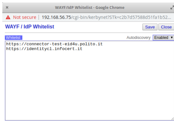
Figure 6: Whitelisting of the Italian eIDAS Connector (in our testbed) and the Infocert IdP in Zeroshell captive portal.
