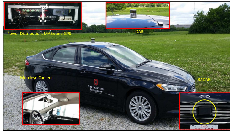
Fig. 1. Autonomous Vehicle Demonstrator at Automated Driving Lab in the Center for Automotive Research of the Ohio State University
