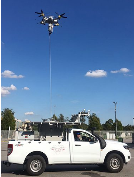
Fig. 1: Tethered UAS by Eagle Sky Light [32]
