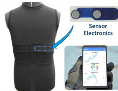
Fig. S5.3. Garment-based sensing of vital signs. Sensors embedded in garments (left and top right) can unobtrusively measure heart rate, respiratory rate, skin temperature, and body motion, and wirelessly transmit information to a smartphone (bottom right) therefore enabling a fine-grained monitoring of individuals affected with or at risk of COVID-19. Courtesy of Cornerstone Research Group, In, OH, USA.
