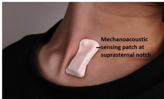
Fig. S5.2. Skin-interfaced wearable sensors. Skin-interfaced sensors allow unobtrusively monitoring physiological information. The Figure S5.2 shows a mechano-acoustic sensing device, allowing to measure coughing, swallowing, and respiration. Such wearable sensors are being applied to patients who have or are at risk of COVID-19. Courtesy of John A. Rogers, Northwestern University, IL, USA [20].
