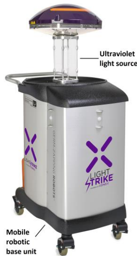
Fig. S5.5. Ultraviolet germicidal irradiation system. Mobile systems with ultraviolet light sources are used to semi-autonomously disinfect areas in hospitals, thereby reducing the risk of viral transmission. Courtesy of Xenex Disinfection Services, San Antonio, USA.
