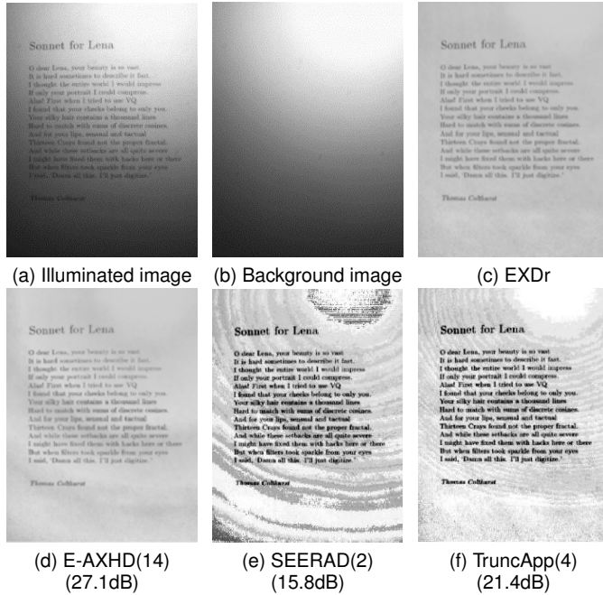
Fig. 12: Background removal using EXDr, E-AXHD, SEERAD and TruncApp.
