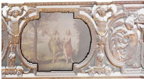
Figure 7. Example of automatic extraction of a planar surface from a LiDAR point cloud using 3DReshaper platform.
