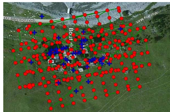
Figure 10. Flight plan (green lines), camera positions (red dots) and measured GCPs (blue crosses) - Zenmuse X4S acquisition.
