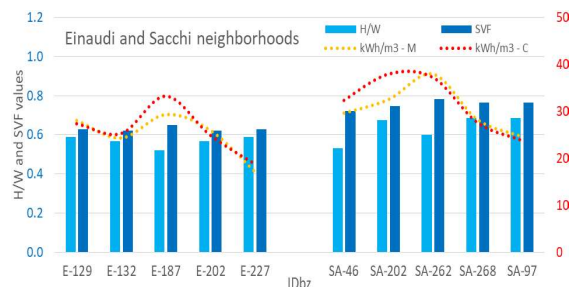
Fig. 10 – Comparison between energy consumption (measured and calculated) and urban parameters for buildings located in Einaudi and Sacchi neighborhoods
