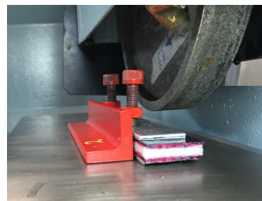
(b) Surface grinder used to refine the beam edges.
