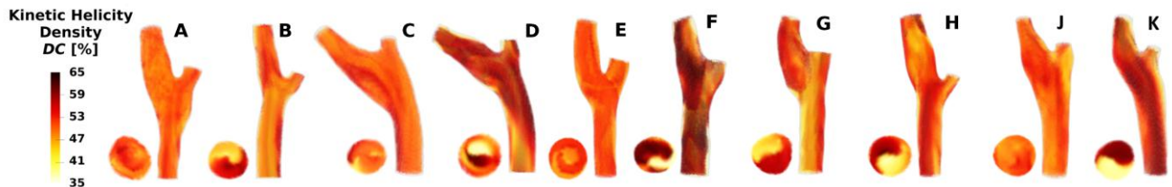
Fig. 11. Volumetric maps of DC for the ten “all-to-all” H_k -based networks. The CCA7 cross-sectional views highlight the existence of two clearly separated low and high DC regions, according to the existence of two distinguishable, counter-rotating, and dynamically correlated helical flow structures.
