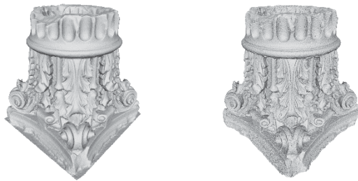
Fig. 2: Photogrammetric models of OBJ2 produced with AMP (left) and P4D (right).
