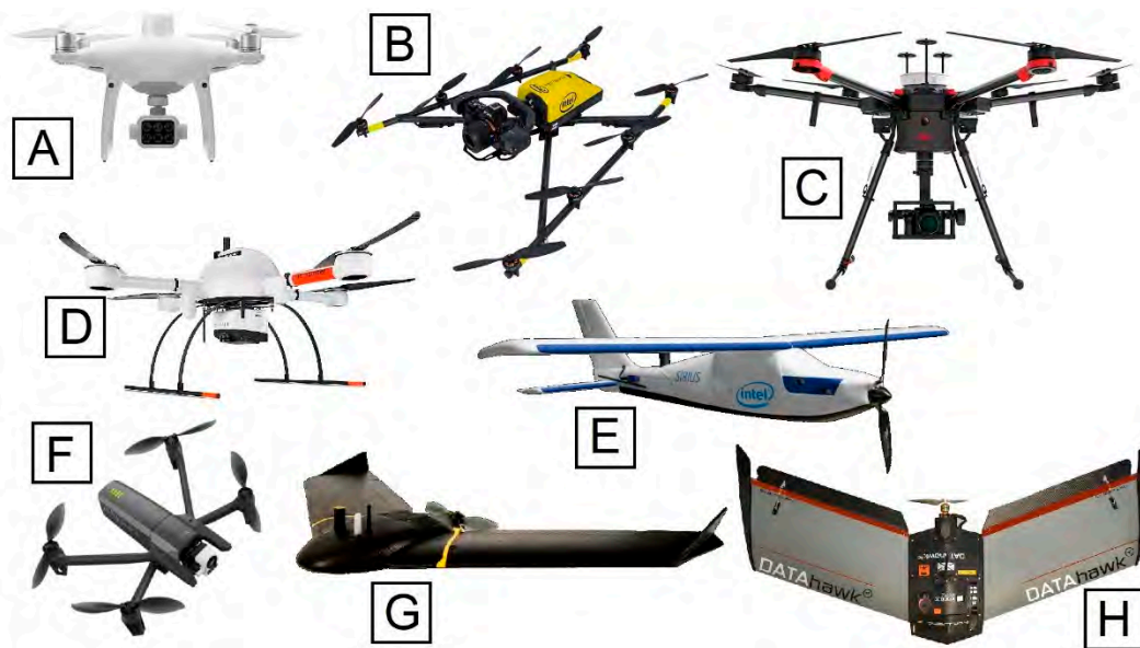
Figure 10. Examples of integrated ready-to-fly UAS: (A) DJI P4 Multispectral; (B) Intel Falcon 8+; (C) Leica Aibot AX20; (D) Microdrones mdLiDAR1000 aaS; (E) Intel Sirius Pro; (F) Parrot ANAFI Thermal; (G) senseFly eBeeX; (H) QuestUAV DATAhawk AG .
