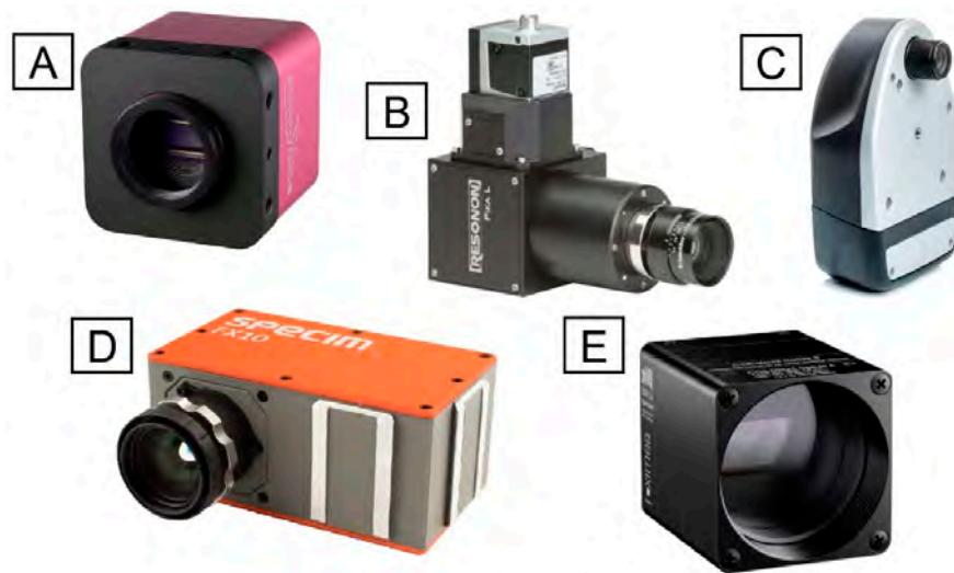
Figure 13. Examples of hyperspectral cameras for UAS: (A) Photonfocus MV1-D2048x1088-HS05-G2; (B) RESONON Pika L; (C) SENOP HSC-2; (D) SPECIM FX10; (E) XIMEA xiSpec Series.
