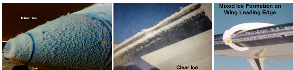
Figure 1. Ice types: rime ice, clear ice, and mixed-ice. (Photo credit: NASA, adapted from [8]).
