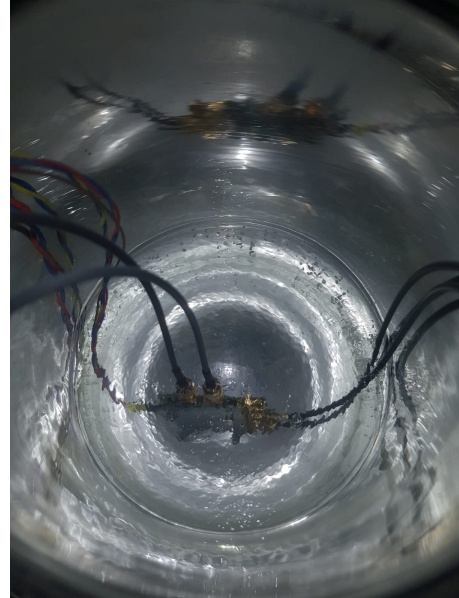
(b) Liquid nitrogen bath to create cryogenic environment
