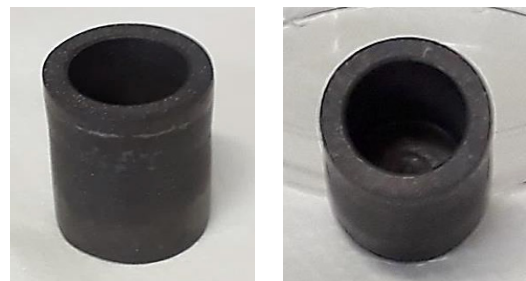
Figure 1. \text{MgB}_2 cup fabricated by spark plasma sintering, drilling and final refining on a lathe machine. Geometrical parameters: outer radius, R_o = 10.15 mm, inner radius, R_i = 7.0 mm, external height, h_e = 22.5 mm, internal depth, d_i = 18.3 mm.
