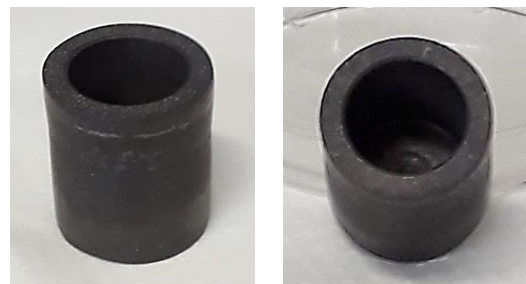
Figure 1. \text{MgB}_2 cup fabricated by spark plasma sintering, drilling and final refining on a lathe machine. Geometrical parameters: outer radius, R_o = 10.15 mm, inner radius, R_i = 7.0 mm, external height, h_e = 22.5 mm, internal depth, d_i = 18.3 mm.
