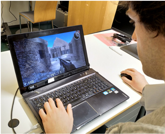
Fig. 11. Experimental setup showing the Tobii 4C eye-tracker (bottom of the screen), peripherals and the Lenovo Y580 client device rendering AssaultCube on the Desert map.
