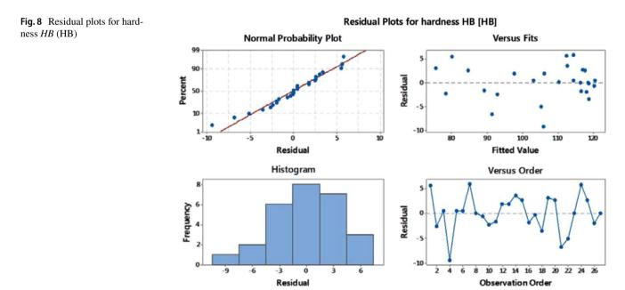
order plot reveals that non-random error, especially of timerelated effects, may be present. The  $R^2$  value is a measure of goodness of fit of the model. It shows that the variation in the response explained by the model describing the relationship between the process variables and the Brinell hardness is 92.3%. Even the predicted  $R^2$  value is very high, reaching 85.9%, suggesting a great predictive capability of the model.
