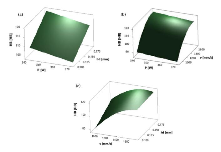
**Fig.9** Surface plot of hardness *HB* (HB) versus: **a** hatching distance  $h_d$  (mm) and laser power *P* (W) (scan speed v was set to 1300 mm/s); **b** scan speed v (mm/s) and laser power *P* (W) (hatching distance  $h_d$
