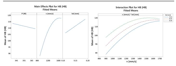
Fig. 7 Main effects plot and interaction plot for hardness HB (HB)
