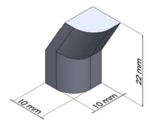
Fig. 5 Samples geometry
