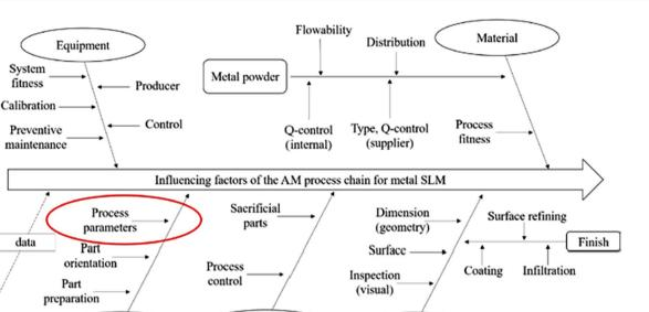
Fig. 3 Ishikawa diagram: influencing factors within AM process chain for SLM. Adapted from Schmidt et al. [19]
