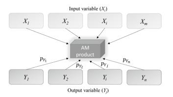
**Fig. 1** Schematic of AM process with *m* input variables and *n* output variables measured on the AM product, with relative probabilities of occurrence of defects  $(p_{Y_i})$
