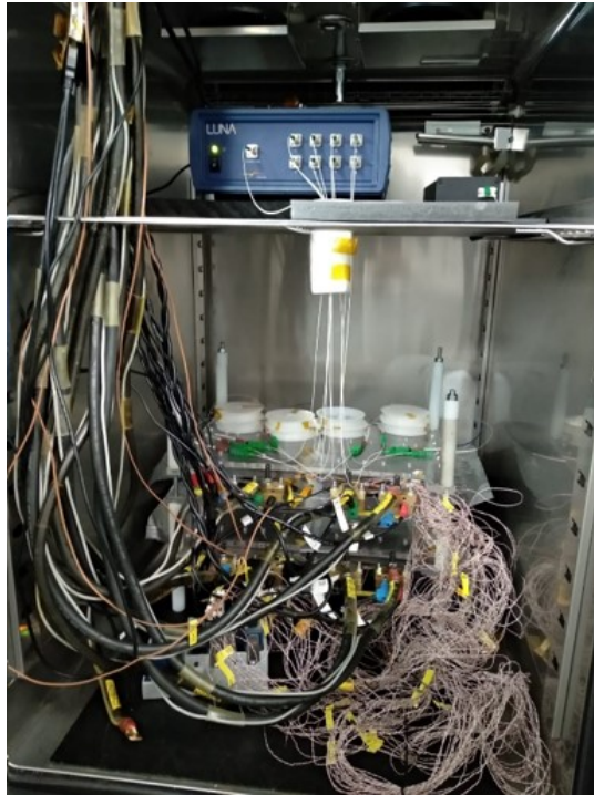
FIGURE 6.1: Testing setup: climatic chamber, cells cycler, distributed fibre optic sensors interrogator, thermocouples.
