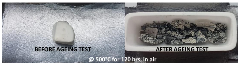
Figure 4.2-23: Ceramacoat™ 512-N coated \text{Mg}_2\text{Si}_{0.487}\text{Sn}_{0.5}\text{Sb}_{0.013} before and after the ageing test in oxidative atmosphere at 500°C for 120 hrs
