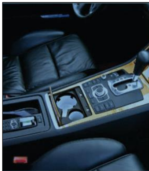
Figure 1.2-5: Peltier elements can keep drinks fresh in thermal cup holders.
