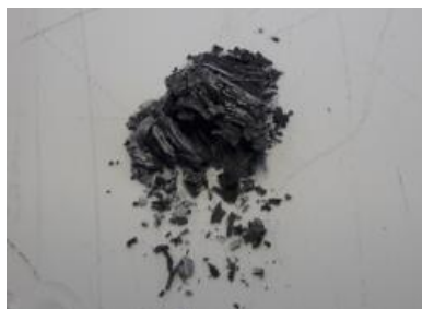
Figure 4.2-4: \text{Mg}_2\text{Si}_{0.487}\text{Sn}_{0.5}\text{Sb}_{0.013} after oxidation test at 500°C for 120 hrs in air without coating
