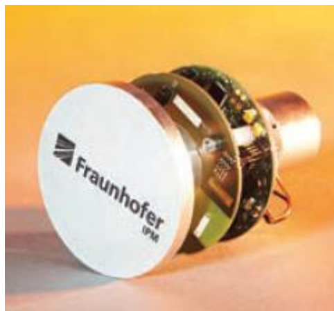
Figure 1.2-3: Thermoelectric sensor. Source: Fraunhofer IPM, Kai- Uwe Wudtke
