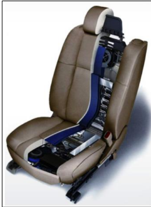
Figure 1.2-6: Cooler for the front seats of a car. Source: General Motors
