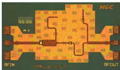
Fig. 30. W-band PA using a 250-nm InP DHBT ( 1.08 \times 0.68 \text{ mm}^2 ) [162] ©IEEE 2017.
