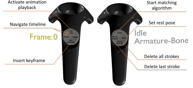
Figure 3: Functionalities available through the controllers.
