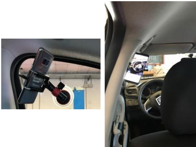
Figure 9. Typical smartphone installation on a car: mobile phone fixed to the driver's front window via a suction holder (left), smartphone position and orientation in the car cabin (right).
