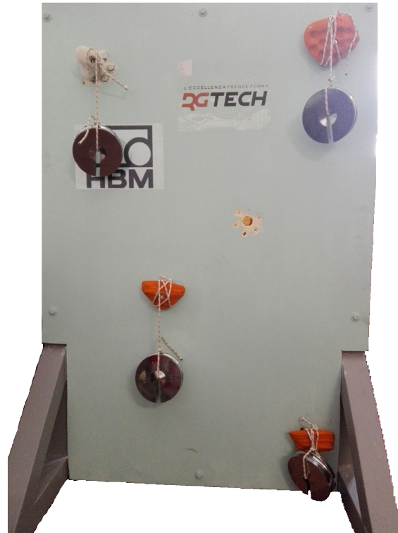
Figure 4: Testing wall with a 50 N weight hanged on each hold
