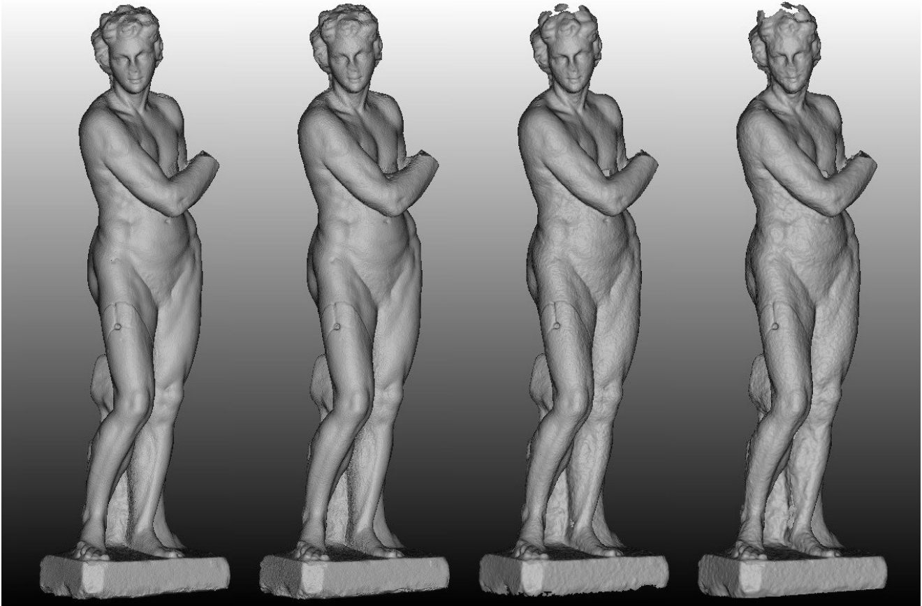
Fig. 3 Photogrammetric models, statue from the Fountain of Hercules (from left to right): AMP VIS, AMP NIR, FZA VIS, FZA NIR
