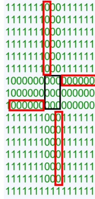
Fig. 2. Bitmap representation of the intersection: queue position in red, intersection area in black.
