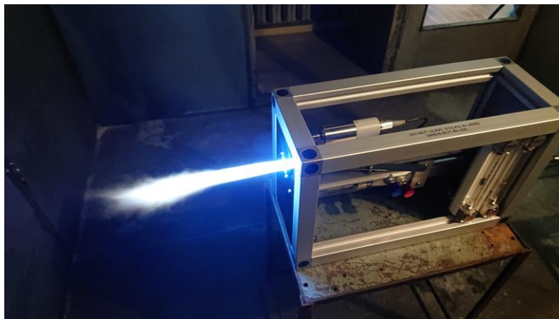
Figure 6 Picture of the nanoaerosol thermal generator in operation
