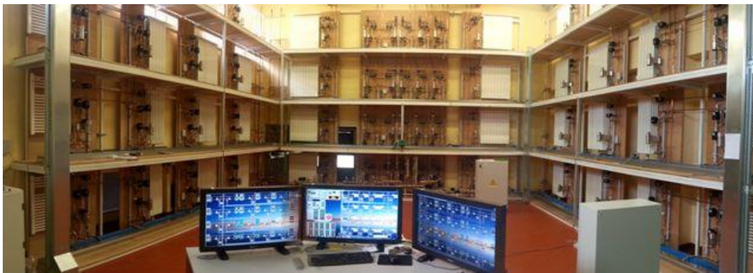
182 Figure 3 - Heat accounting experimental mockup at INRIM
