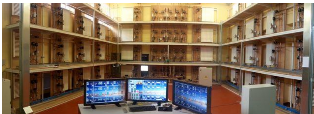
182 Figure 3 - Heat accounting experimental mockup at INRIM
