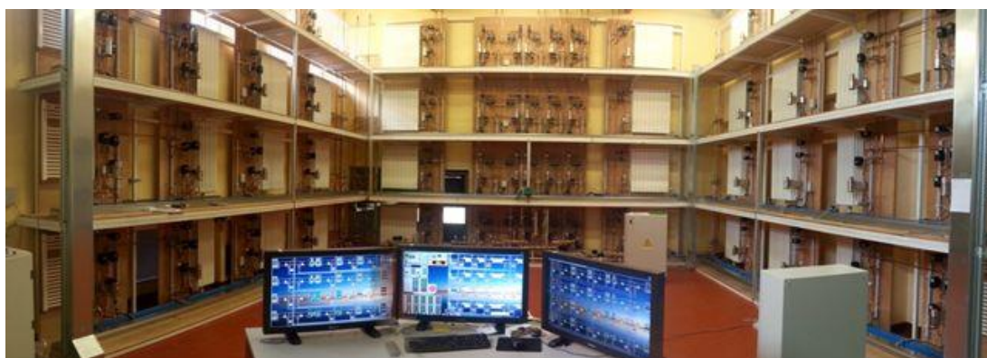
182 Figure 3 - Heat accounting experimental mockup at INRIM
