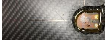
Figure 15: Bonding of circular piezo patch to the composite plate with epoxy resin, as recommended by PI (b).
